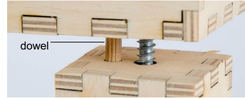
Figure 22: PÅCKER allows preventing rotation by inserting a dowel parallel to single screw connectors.
