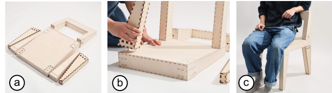
Figure 7: Figure 7: (a) The user unpacks the decomposed chair, (b) assembles the components with the connectors. (c) The resulting chair is load-bearing.
