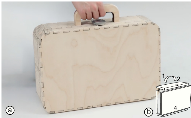
Figure 14: (a) A laptop case based on dovetail joints. (b) Dovetail joints close the chain that connects the bottom to the handle.
